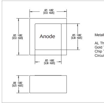
Metallization: Top: (anode) AL Back: (cathode) Au
