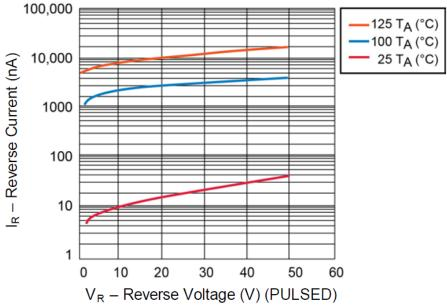
FIGURE 4 1N5711 Typical Variation of Reverse Current ( $I_R$ ) vs Reverse Voltage ( $V_R$ ) at Various Temperatures
