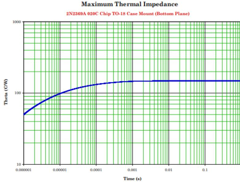
FIGURE 12. Thermal impedance graph (TO-18 TO-46) ( $R_{\theta JC}$ ) for 2N2369A.
