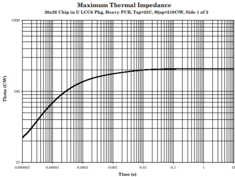
FIGURE 13. Thermal impedance graph ( $R_{\theta JSP}$ ) for 2N2369AU and 2N3227U.
