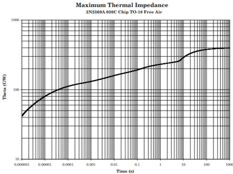
FIGURE 11. Thermal impedance graph (TO-18) ( $R_{\theta JA}$ ) for 2N2369A and 2N3227.
