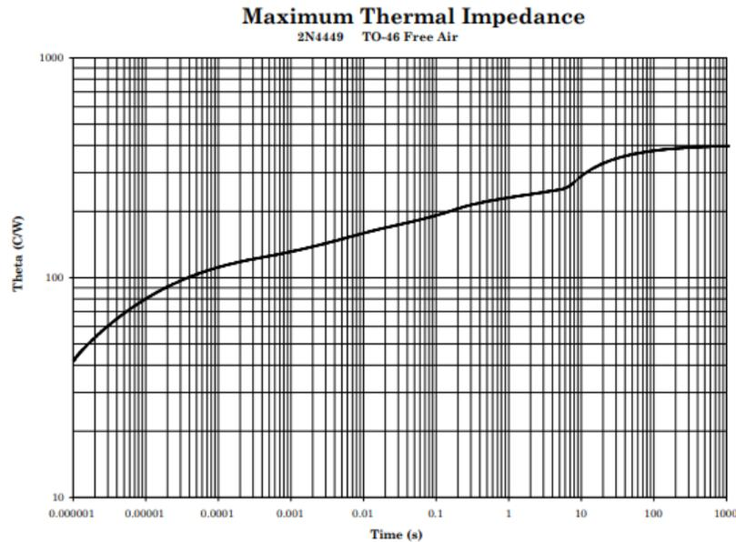
FIGURE 10. Thermal impedance graph TO-46 ( $R_{\theta JA}$ ) for 2N4449.
