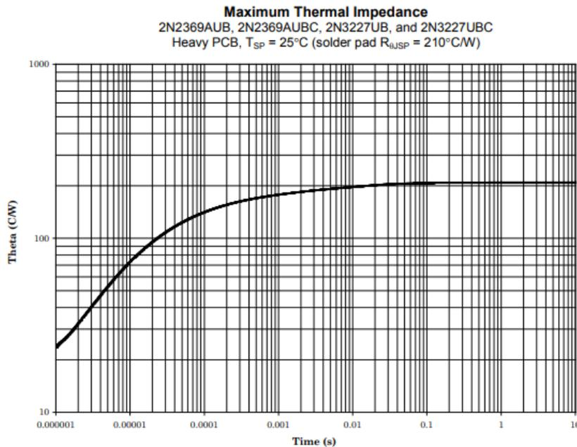
FIGURE 9. Thermal impedance graph ( $R_{\theta JSP}$ ) for 2N2369AUB, 2N2369AUBC, 2N3227UB, and 2N3227UBC.
