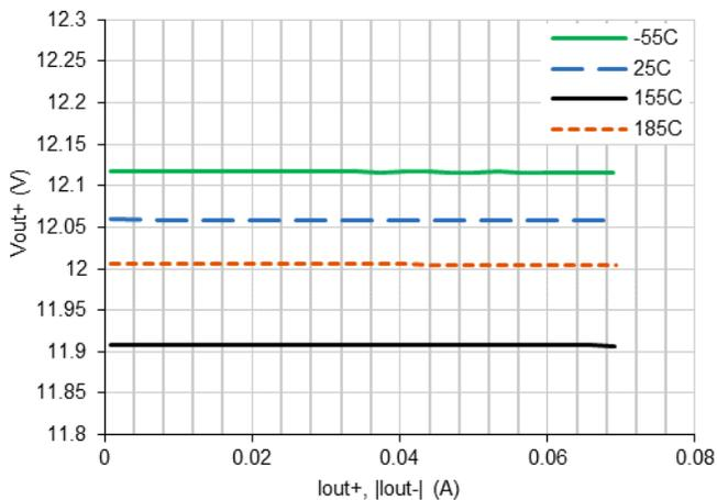
4.1.6 HTD1R5N-2812D Output Voltage vs. Current
