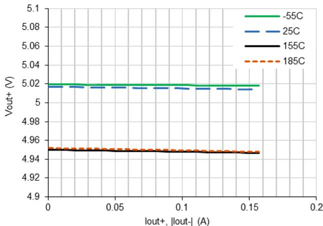
4.0.6 HTD1R5N-2805D Output Voltage vs. Current
