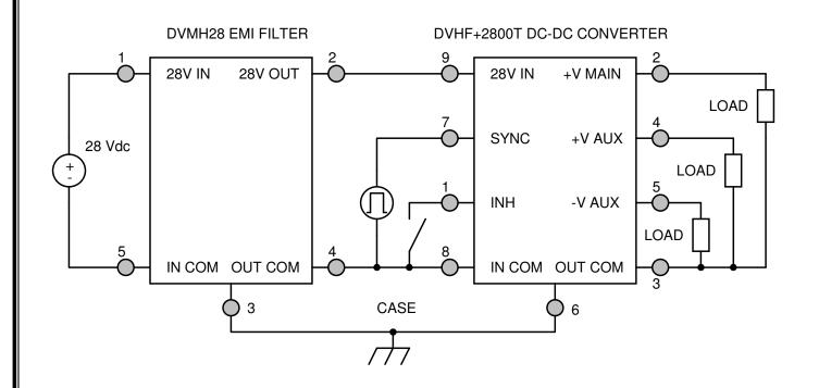
Figure 6 - Converter with EMI Filter
