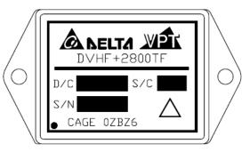
Figure 1 – DVHF+2800T / DVHF+2800TF DC-DC Converter (Exact marking may differ from that shown)
