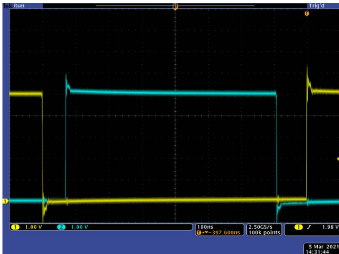
Figure 5. FBS-GAM02 POL Evaluation Board BIN-TIN and TIN BIN Logic Input Dead Time
