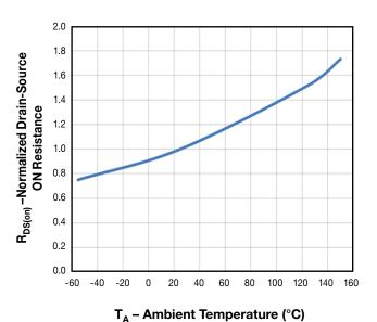
Figure 9. Typical Normalized Drain-Source ON Resistance vs. Ambient Temperature
