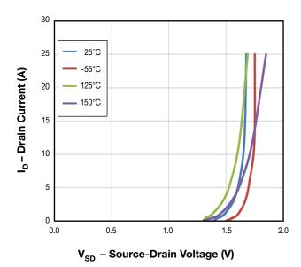
Figure 8. Typical Source-Drain Voltage vs. Temperature
