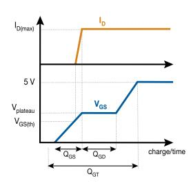
Figure 15. Typical Gate Charge Test Waveform
