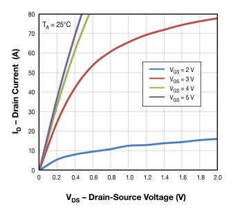
Figure 5. Typical Output Characteristics
