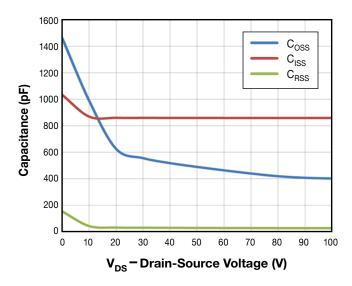
Figure 10. Typical Inter-Electrode Capacitance vs.
