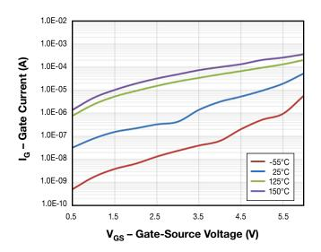
Figure 2. Typical Gate-Source Leakage Current vs. Ambient Temperature
