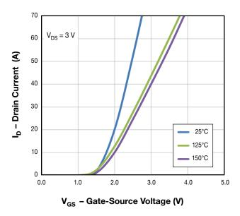
Figure 4. Typical Transfer Characteristics  $(V_{DS} = 3V)$
