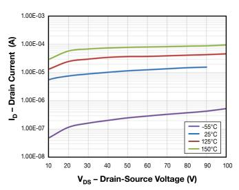
Figure 3. Typical Drain-Source Leakage Current vs. Ambient Temperature
