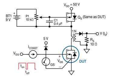
Figure 14. Charge Test Circuit
