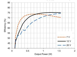
4.0.6 HTD1R5N-1205D Output Voltage vs. Current
