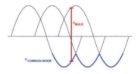
Figure 5. Diagram of 3-phase AC waveforms.
