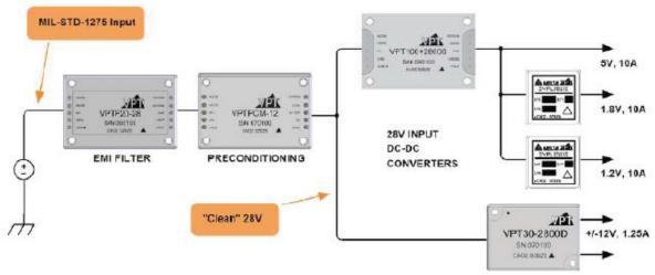
Figure 1. MIL-STD compliant 28V input power supply.
