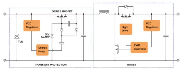
Figure 2. Input Voltage Conditioning Circuit.
