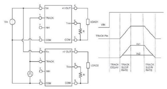
Figure 3. Tracking waveforms.
