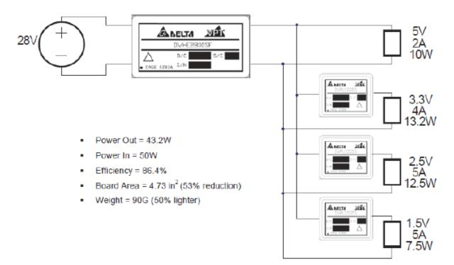
Figure 2. Point of load system approach
