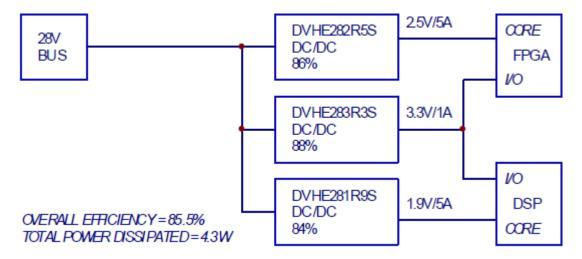
Figure 2. Low Voltage Application Using the DVHE2800S Series.
