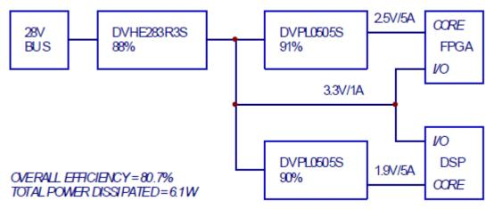
Figure 5. Low Voltage Application Using the HERO Power System.
