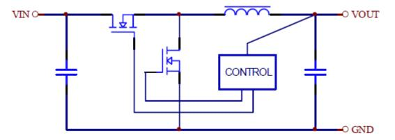
Figure 4. Non-Isolated Synchronous Buck Schematic.
