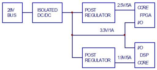
Figure 3. Low Voltage Application Using Post Regulators.
