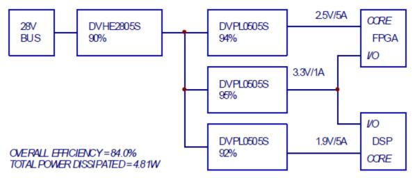
Figure 6. Low Voltage Application Using the HERO Power System Distributed 5V Bus Approach.
