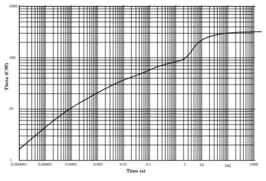
TA = +25°C at Pdiss = 500mW (Thermal Resistance ReJA = 325°C/W at 500mW)
